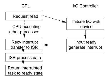
Interrupt service can be complicated on modern machines – consider pipelined execution (see text).
