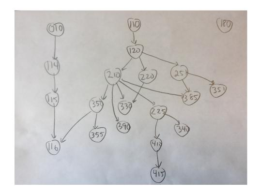
One algorithm to compute a topological sort of a dag is based on a depth-first traversal of the graph is described in the text.
