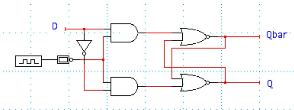
This is the *Clocked D-type Flip-Flop*.
