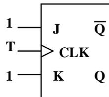
The input  $T$  is so-named because it will toggle the outputs.
