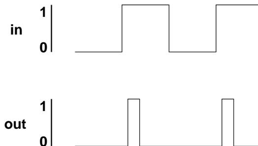
The length of time that the output is 1 after the switch of the input from 0 to 1 depends on the gate delay of the inverter.
