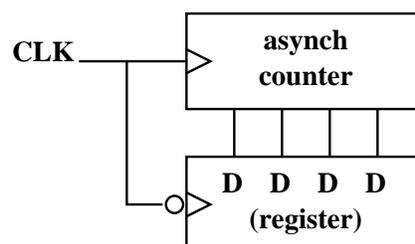
The values can come out of the top counter asynchronously, but we don't put them into our register until the clock goes back down.
