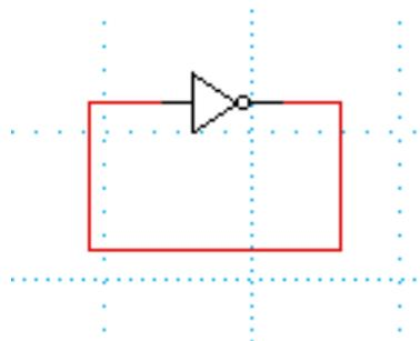
The electrons can go around the wire from the output back to the input very quickly – something around half the speed of light, maybe more.
