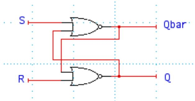
At any given time, it has a stable value when  $S$  and  $R$  are 0.
