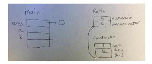
When the constructor returns, two things happen: its memory for parameters and local variables goes away, and it returns the reference to the new object's instance variables. In our case, we're storing that reference in main's local variable a.
