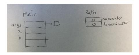
Our Ratio class has two instance variables of type int, named numerator and denominator. Java automatically initializes all instance variables with zero, false, or null values, as appropriate. So our int variables get 0.
