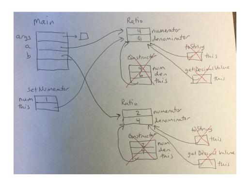
We have a slot for the formal parameter num, initialized to the value of the actual parameter, 1. Then the this reference, initialized to the object, which is the thing that comes before the . in the call.
