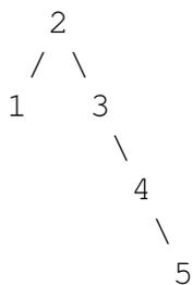
Again, we need to fix the balance condition. Here, we can apply one of these rotations on the right subtree of the root:
