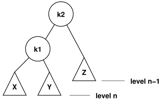
After an insert, the subtree  $X$  increases in height by 1:
