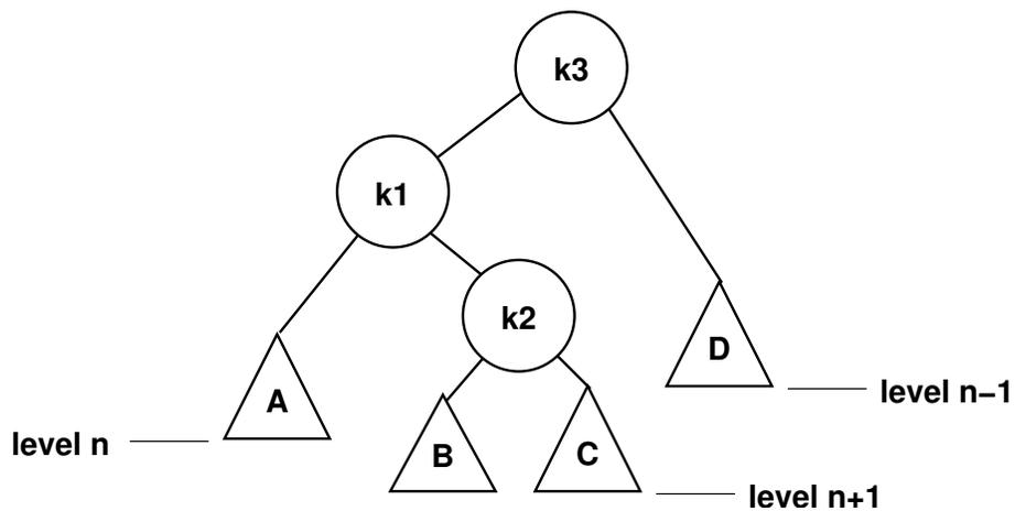
Here, only one of  $B$  or  $C$  is at level  $n + 1$ , since it was a single insert below  $k_2$  that resulted in the AVL condition being violated at  $k_3$  with respect to its shorter child  $D$ .
