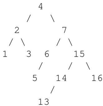
What do we have here? Looking up from the insert location, the first element that violates the balance condition is the root, which has a difference of two between its left and right child heights.
