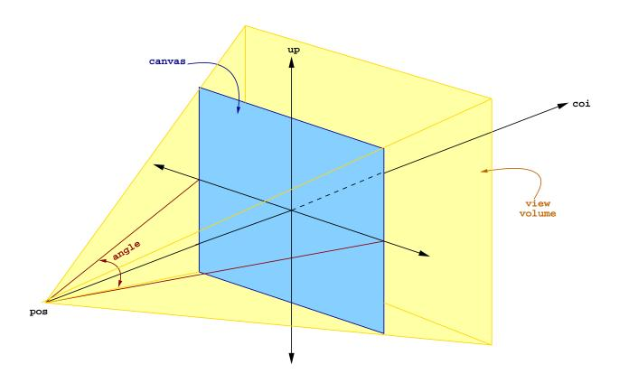
The yellow shaded pyramid in this figure (which extends back infintely) is the *view volume*, and the objects we see are everything in the view volume that is not occluded by an object between it and the camera position (called its *viewpoint*). The blue rectangle, labeled the "canvas", is the intersection of the view volume with the *image plane*.
