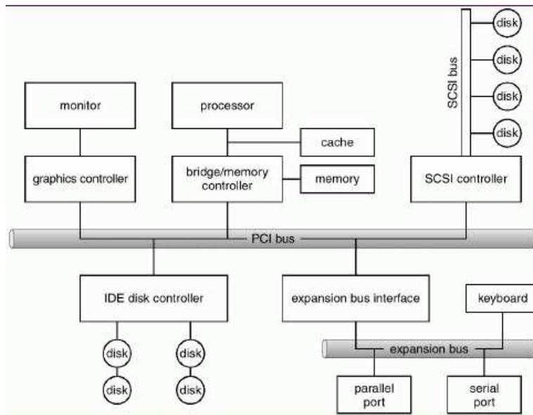
Note the presence of *device controllers* – hardware that connects directly to the main bus on behalf of actual devices.
