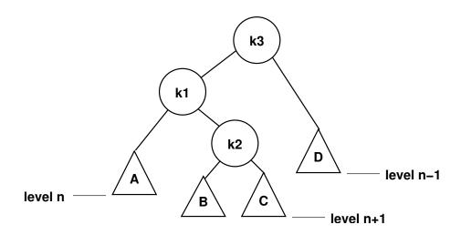
Here, only one of B or C is at level n+1, since it was a single insert below  $k_2$  that resulted in the AVL condition being violated at  $k_3$  with respect to its shorter child D.
