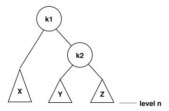
For this insertion type (left subtree of a left child – case 1), this rotation has restored balance.
