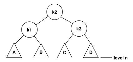
We're essentially rearranging  $k_1$ ,  $k_2$ , and  $k_3$  to have  $k_2$  at the root, and dropping in the subtrees in the only locations where they can fit.
