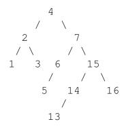
What do we have here? Looking up from the insert location, the first element that violates the balance condition is the root, which has a difference of two between its left and right child heights.
