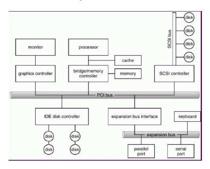
Note the presence of *device controllers* – hardware that connects directly to the main bus on behalf of actual devices.
