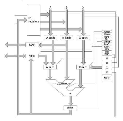
Figure 1: The extended microarchitecture used for the WC34000.
