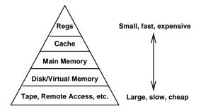
We have already considered how the use of registers is different from main memory, in particular for the MIPS ISA, where all computation must operate on values from, and store results in, registers.
